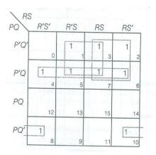
There are three Quads and 1 Pair: Quad 1 ( $m_1 + m_3 + m_5 + m_7$ ) reduces to *P'S* Quad 2 ( $m_4 + m_5 + m_6 + m_7$ ) reduces to *P'Q* Quad 3 ( $m_2 + m_3 + m_6 + m_7$ ) reduces to *P'R*
