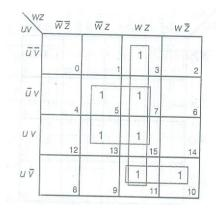
There are 2 Quads and 1 Pair: Quad 1 ( $m_3 + m_7 + m_{11} + m_{15}$ ) reduces to wz Quad 2 ( $m_5 + m_7 + m_{13} + m_{15}$ ) reduces to vz Pair 1 ( $m_{10} + m_{11}$ ) reduces to u v wHence, the final expression is: F(u, v, w, z) = w z + v z + u v w
