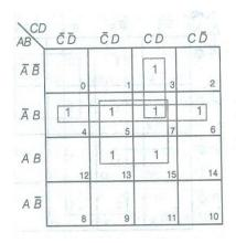
There are 2 Quads and 1 Pair: Quad 1 ( $m_4 + m_5 + m_6 + m_7$ ) reduces to *AB* Quad 2 ( $m_5 + m_7 + m_{13} + m_{15}$ ) reduces to *BD* Pair 1 ( $m_3 + m_7$ ) reduces to *ACD* Hence, the final expression is: F(A, B, C, D) = AB + BD + ACD
