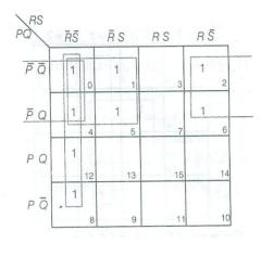
There are 3 Quads: Quad 1 ( $m_0 + m_4 + m_8 + m_{12}$ ) reduces R S Quad 2 ( $m_0 + m_1 + m_4 + m_5$ ) reduces P R Quad 3 ( $m_0 + m_2 + m_4 + m_6$ ) reduces S P Hence, the final expression is: F(P, Q, R, S) = RS + P R + S P
